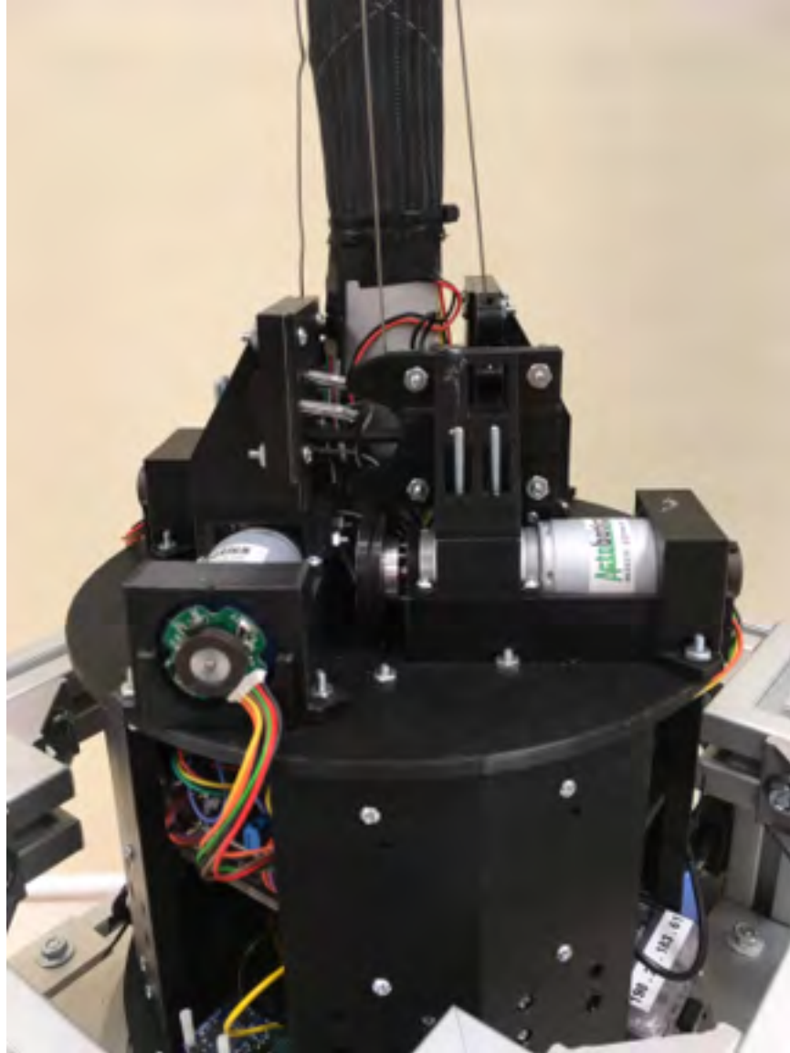
Figure 3.10: The motor plate which is mounted to the top of the central structure. Here is where the tendon motors are mounted with the tension sensors and the spools to wind the tendons and measure length.
