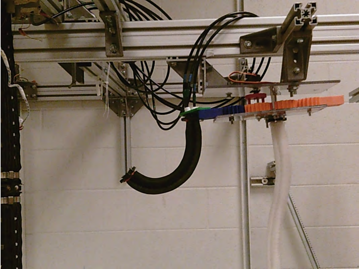
Figure 4.1: An example of a single section extensible continuum robot [2].
